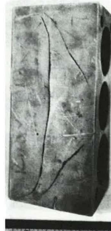
Figure 11. The design of this forming die, made of Type W1 tool steel, presents an almost impossible problem to the heat treater. Because of the blind holes and the thin section between them, the die cracked during heat treatment. Unless the die can be totally redesigned, the use of an air-hardening steel is imperative (Bethlehem Steel Corporation).
